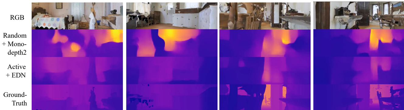
Fig. 4: Depth Prediction Visualization. Our proposed approach demonstrates better accuracy and consistency in producing depth maps compared to the conventional random exploration strategy with Monodepth2. This can be attributed to the enhanced exploration capabilities of our active policy, which also leverages multi-frame inputs to effectively overcome limitations associated with single-frame inputs.
